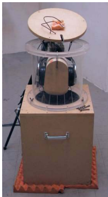
Figure 8. Dummy head with “flat-plate” microphone in a volume suitable for relatively high noise levels (130 dBA).
