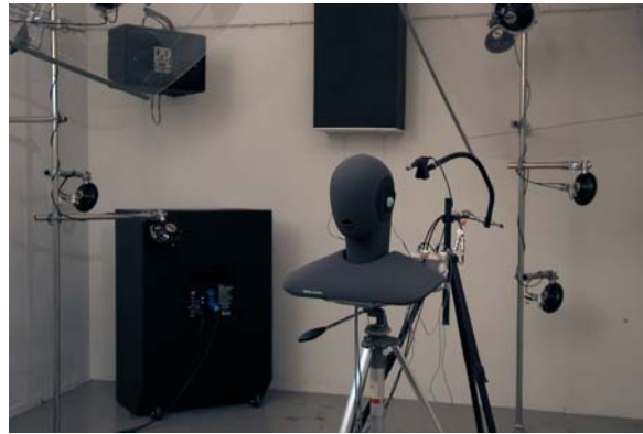
Figure 7. Artificial head placed in a high noise room, designed for generation of a diffuse sound field (max. 120 dBA). Two of the five high power loudspeakers (back view) are visible at the left. In the center of the wall a sound absorption module is placed. The small loudspeakers are not used (these are available for REAT experiments).
