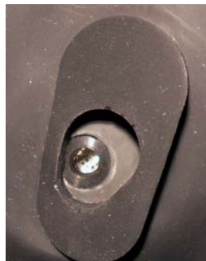
Figure 6. Artificial ear mounted in an artificial head (MIArtE).
